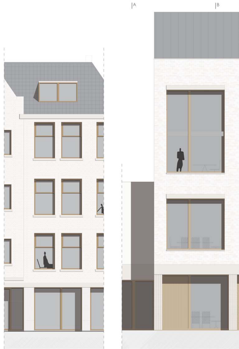
16 Il: facade fragment south facade, renovation daycare, Ir: facade fragment south facade, new building part, rl: 1:20 details (b), rr: 1:20 details (a)
